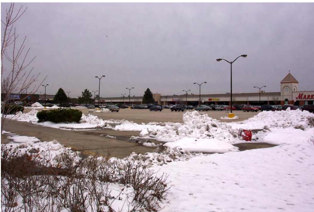
Figure 3-16 Westside Plaza Expansive Parking Area Increases Off-Site Runoff Volume
